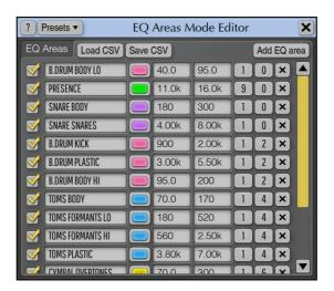
This window allows you to define your own highlight areas on the spectrum display. Highlighted areas can be used as helpers to remind you of the signal types present in specific frequency ranges.
